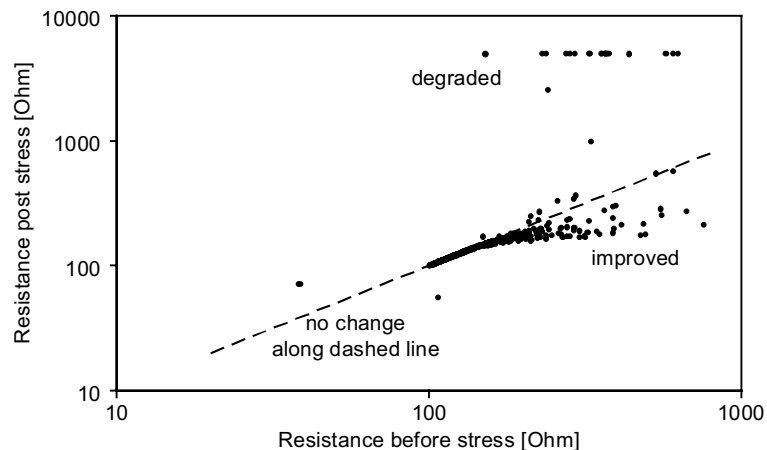
Fig. 20. Relation between structure resistance before and after constant current stress. The bad structures are due to open contacts in which the barrier layer conducts all current. The improved resistance of test structures reflects a breakdown of some residual insulating layer in the bottom of the contact hole.
