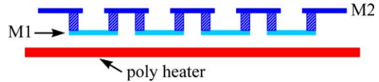
Fig. 21. Schematic cross-section of a self-heated via chain test structure. The poly-Si strip heats the structure above and accelerates the degradation.
